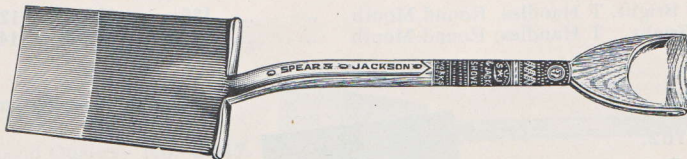
No. C160A. Scotch Pattern. S. & J.'s "Mermaid" Brand, Solid Strapped, extra quality Ash Handles, Flat Tread, not Ribbed, 12" Straps, 3 Rivets.
